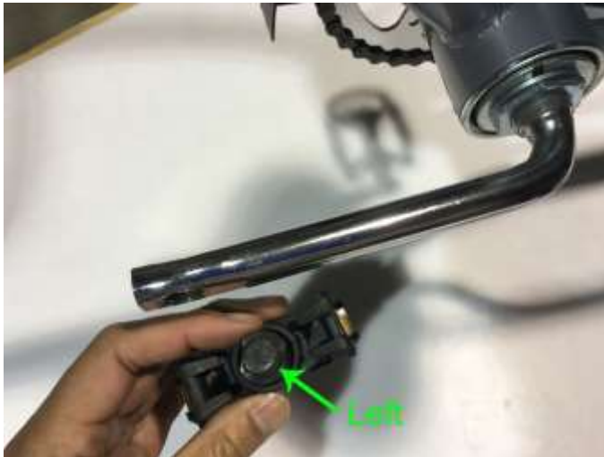
029 - Thread Counter-clockwise direction
