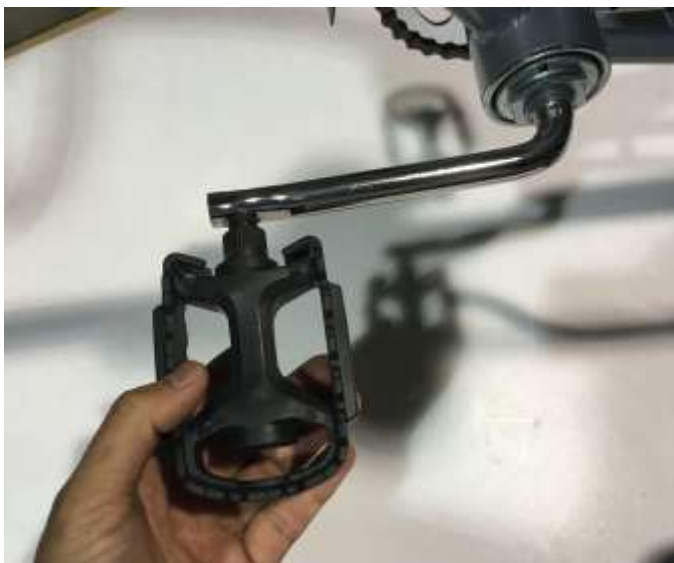
029 - Thread Counter-clockwise direction
